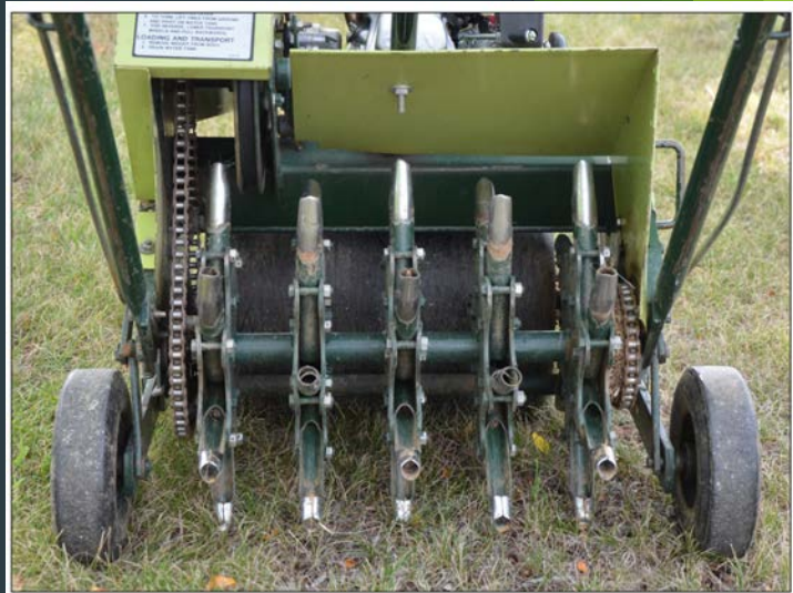
Figure 5. A common lawn aerifier available at rental agencies. This roller-type aerifier inserts tines as it rolls along.
