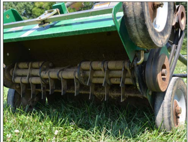
Figure 2. A good dethatching machine has fixed knives or sling blades; spring tines are not effective.
